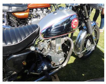
This one was a doozy. Mixed ZB barrel and head (die and sandcast), '49 ZB bottom, mid-'50s g'box and most of the rest, except for a late '60s twin-leader front brake!
